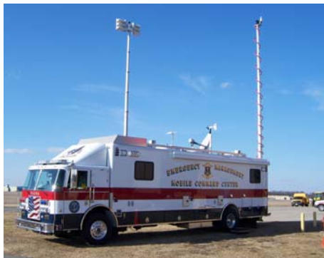
MCC With Mast Camera and Light Tower Deployed
